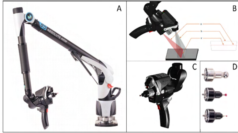
Figure 3.5: (A) Romer Absolute Arm, (B) Laser Scanner, (C) Contact Probe, and (D) Contact probe variety
