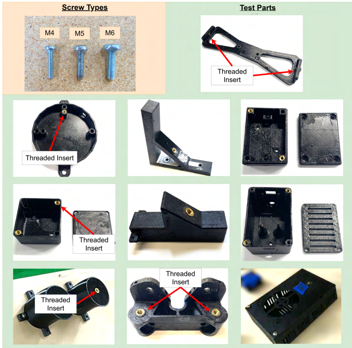
Figure 8.10: Left: The three Screw Types (M4, M5, and M6) used for the trials and Right: The ten test parts selected for performing screwdriving trials. Each of them has a different geometrical complexity, size, and shape, and they are representative of different industrial settings (E.g., Electrical Components, Automobile Parts, Refrigerator Parts, etc.). Furthermore each of them have different screw types and at different orientations to simulate a realistic HMLV scenario
